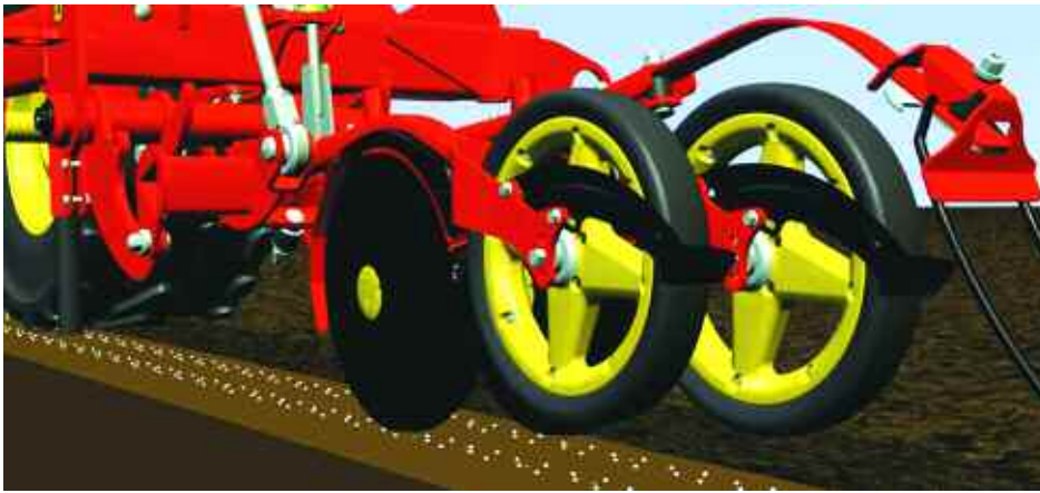
Modern combined drills typically place fertiliser in a narrow band close to the seed
